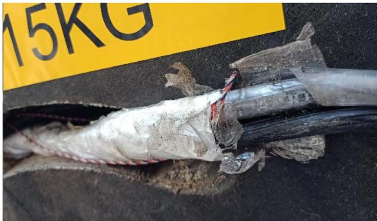
The manufacturer and supplier were contacted, who informed Standards Engineering that the string was used for internal factory processes and should have been removed prior to supply to Power and Water.
