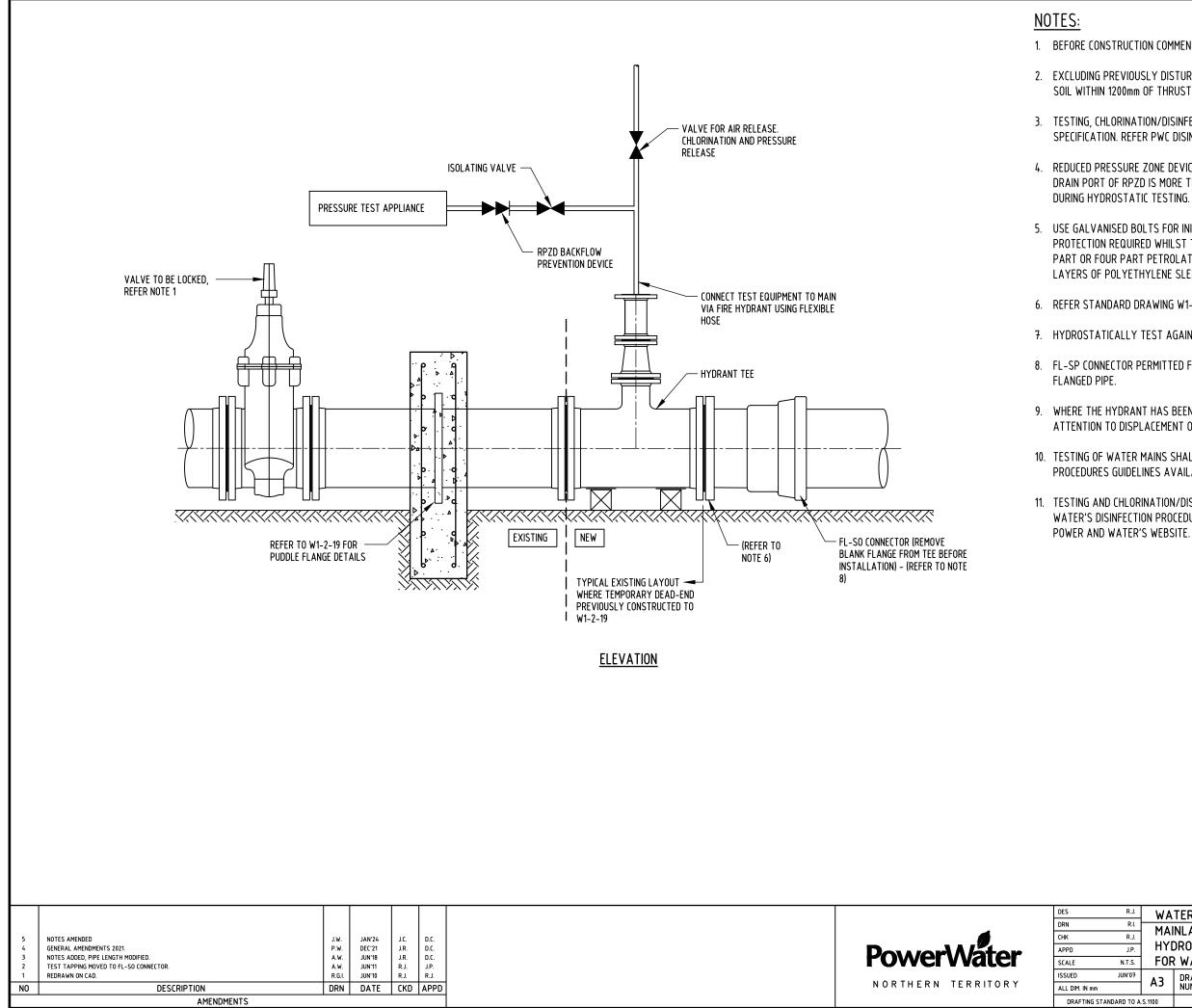
1. BEFORE CONSTRUCTION COMMENCES, VALVE TO BE LOCKED IN CLOSED POSITION BY PWC.
